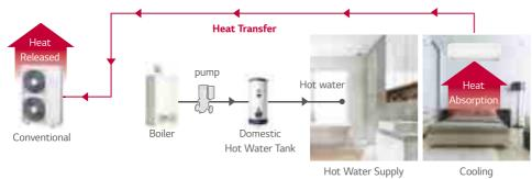
Absorbed heat from indoor space is used for making hot water.
