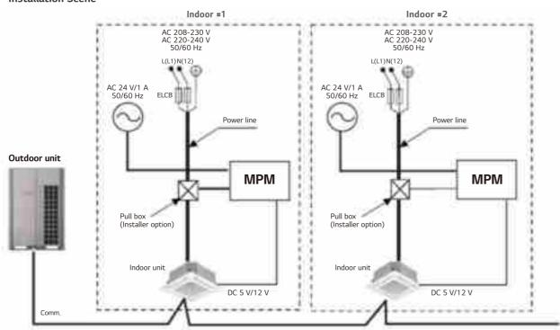
When Multi-tenant Power Module is adopted, CN-EXT must used for it. Instead of being used CN-EXT, PDRYCB000 (220Vac input) / PDRYCB100 (24Vac Input)
