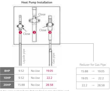
$\ensuremath{\mathbb{X}}$  For using as Heat Pump, Reducer for Gas pipe should be used. Reducer is included in outdoor unit.
