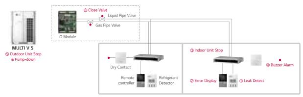
% If the concentration of the refrigerant in the air exceeds 6,000 ppm more than 5 seconds, the function will be activated. (Refer to operation sequence which written in red, 1-6)
