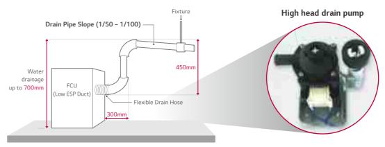
\* All of LG's FCU's have a high head drain pump built in.
