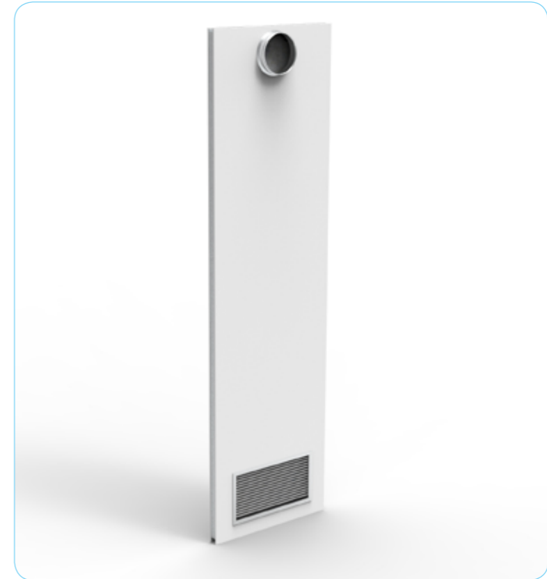
Exhaust panel The exhaust wall panel is special type of panel with a built-in exhaust grille in the lower part of the wall and a horizontal cylindrical connection at the top of the wall. This wall panel is intended for installation in areas where there is not enough space to install a classic vertical duct and the air from the room is provided through the wall panel. A cylindrical connection channel is connected to the technical zone above the ceiling. Standard panel wall options apply to exhaust panel. Dimensions:
